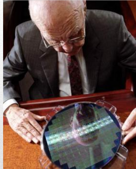
Mr. Kibly in this 2002 photo of a modern 300mm Wafer, with 108 Die/IC, each with thousands of Transistors!
